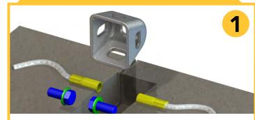
Align prefabricated concrete sections, insert turnbuckle into recess making sure to align anchors to turnbuckle openings.
