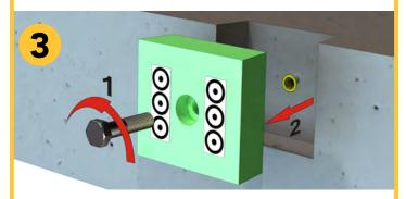
After concrete has cured, the recess units are removed leaving open recess in formwork to affix the turnbuckle in place to anchor.
