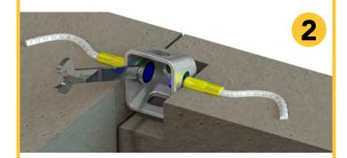
The fastener connections are tightened using a ring ratchet wrench until the optimum joint width is reached.
