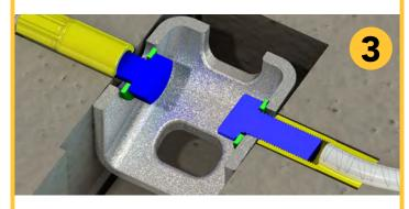
When the prefabricated sections are under tension, the recesses for the tie points can be sealed with appropriate sealing materials and the external recess is ready to be filled.
