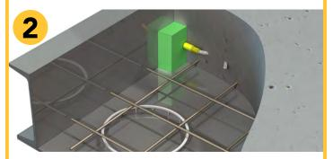
Place the recess unit in appropriate position. By marking the formwork and the recess units, the anchors can be precisely fitted efficiently without extensive measurement. The built-in magnets within the recess unit simplify the placement on the steel table. Place the related anchor fittings and pour in the cement.
